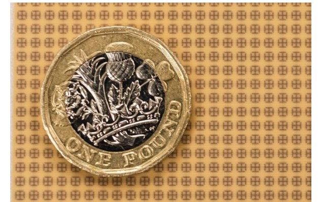
META medical RF metasurface for impedance matching
