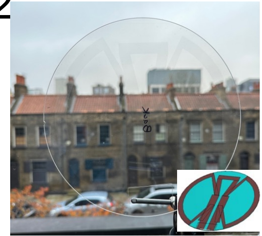
TV antenna patterned on Glass @400-800 MHz
